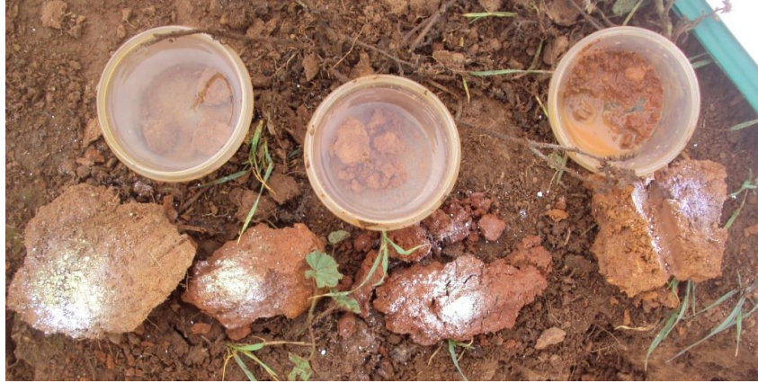
Figure 1. Photograph showing samples from various soil horizons tested for soil pH (water) using the hand test kit. Samples on the left are A 1 and B 1 horizon samples showing acidic soil pH levels.
